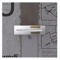
Seal the butt joints of the wedi Subliner Dry membranes with wedi 520 flexible sealant and wedi Tools sealing tape.
