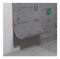
Apply a thin-bed flexible tile adhesive (wedi 320 or similar) with a 4 or 6 mm grooved trowel. Lay the wedi Subliner Dry and press it on with a rubber roller or wooden board.
