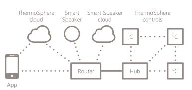
Mesh networking makes sure your thermostats are always connected. Extra connections between each thermostat provide a backup signal if a thermostat should ever lose its connection to the hub.
