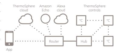
Mesh networking makes sure your thermostats are always connected. Extra connections between each thermostat provide a backup signal if a thermostat should ever lose its connection to the hub.
