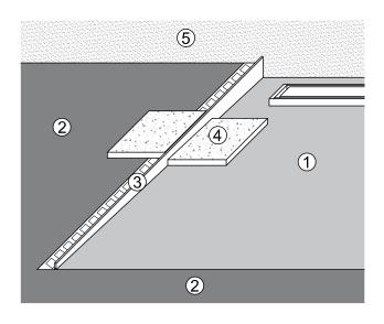
The sloping JACKOBOARD® Aqua Line Profile (available as an accessory) can be inserted between the edge and the screed. The sloping profile is available as a left version (illustrated) or as a right version.
