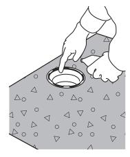
6) Coat the entire underside of the shower element with tile adhesive.
