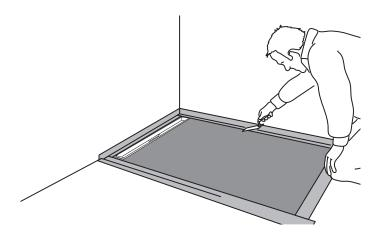
8) All connecting joints are sealed with the JACKO-BOARD® sealing set (or equivalent).
