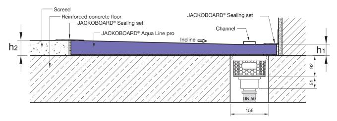
h1 = 48 mm = thickness of shower element (43 mm) + 5 mm mortar (min. height in the channel area)
