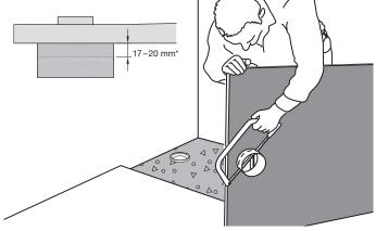
\*12 - 15 mm into the drain bowl + 5 mm bonding mortar
