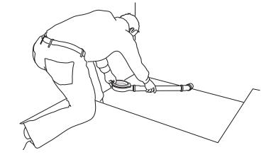
3) The floor recess is filled with levelling screed and smoothed flat. The resulting surface must be flat and horizontal. The height difference to the surrounding floor screed equates to the thickness of the shower element (60, 70, 80 mm) + approx. 5 mm tile adhesive. The floor drain must bond firmly with the mortar to enable load absorption.
