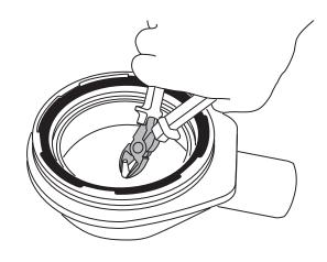
2) Insert the floor drain into the existing DN 50 pipe. Adjust the floor drain to the required height. The required clearance between the upper edge of the floor drain and the upper edge of the surrounding floor screed equates to the thickness of the shower element (60, 70 or 80 mm) + approx. 5 mm tile adhesive. (see the "installation height" sketch on page 7).
