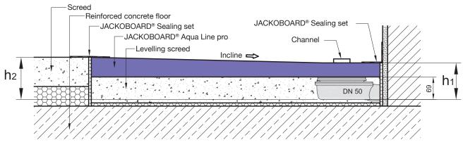
h1 = 114 mm (minimum installation height in the channel area)
