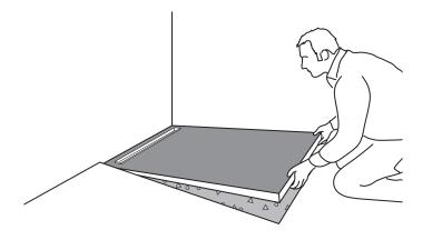
7) Position JACKOBOARD® Aqua Line pro in the screed recess, making sure the drain nozzle on the channel fits into the seal ring on the drain.
