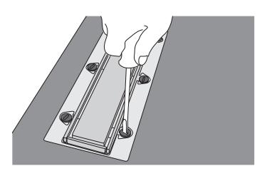
**11)** The stainless steel track can be tiled on the back. Simply turn it over and tile it.
