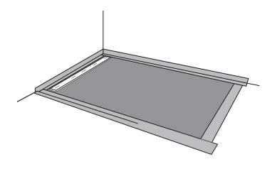
10) The channel is height variable and can be adjusted to different tile thicknesses (6-21 mm). Change the height by adjusting the red screws with a slotted screwdriver.
